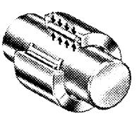
Skewed rollers contact the shaft at one point and the outer race at two points. This causes extremely high contact stresses and bending of the rollers, resulting in unpredictable bearing life. Skewing also induces undesirable thrust loads.
